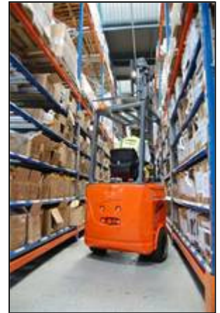
Bendi articulated forklifts can operate in aisle widths of 1.6m
